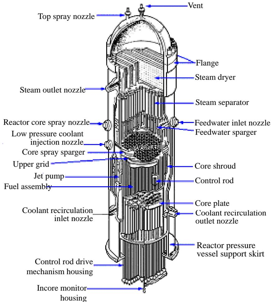
**Figure 3. Internal Structure of BWR Reactor Vessel**
