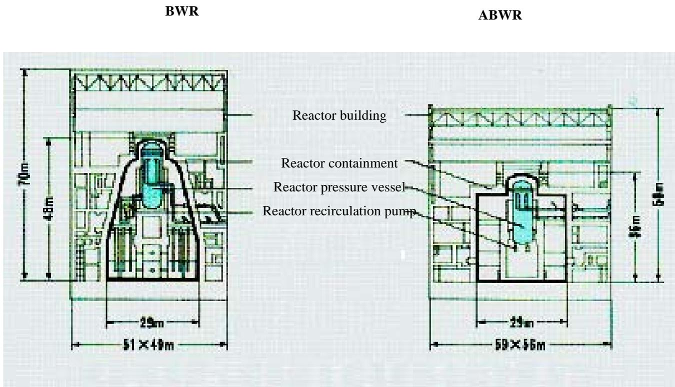
**Figure 16. Reactor Containment for BWR and ABWR**
