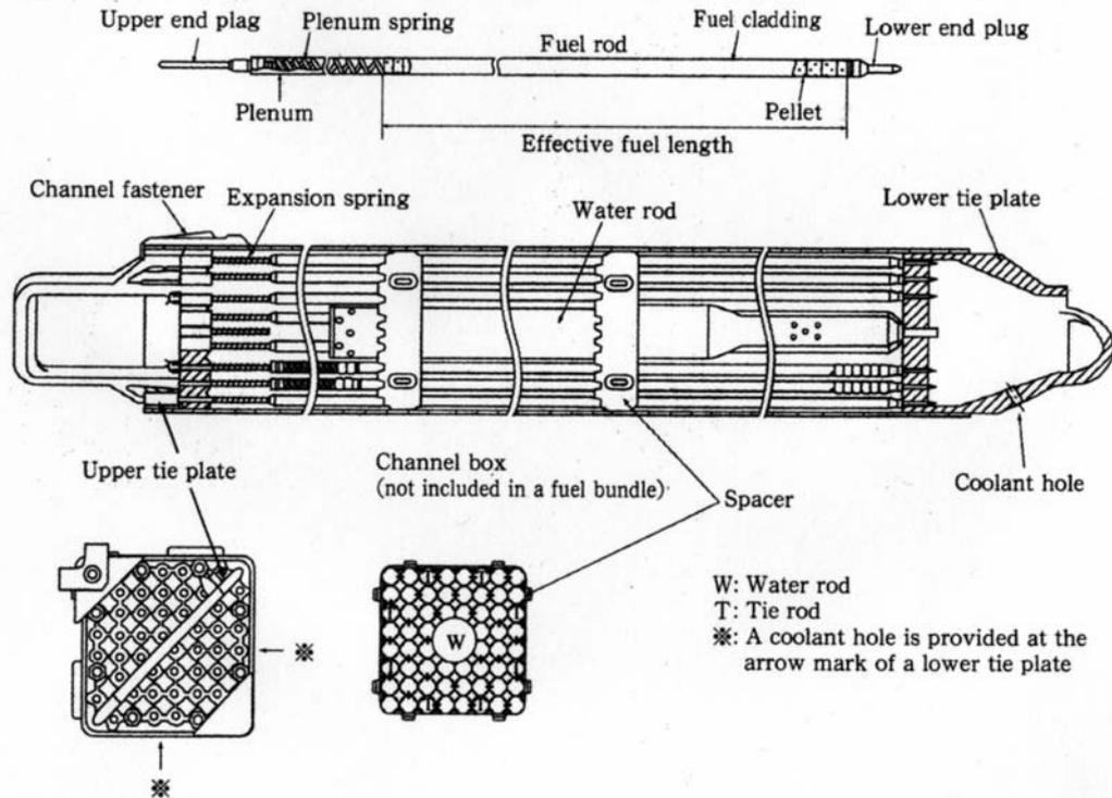
Figure 4. BWR Nuclear Fuel Structure
