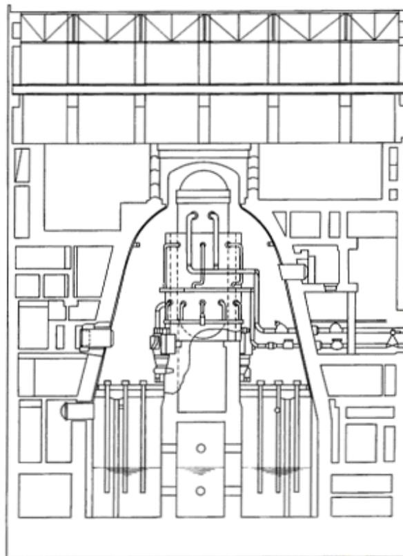
**Figure 7. BWR Containment in the Reactor Building (Improved Mark-II)**
