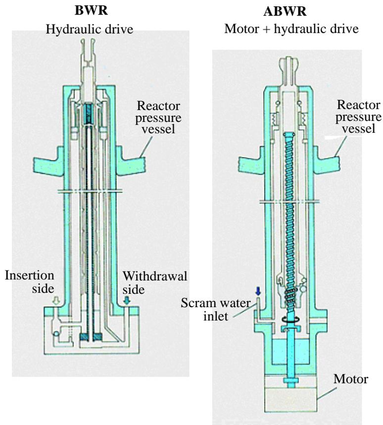
**Figure 13. Control Drive Mechanism for BWR and ABWR**
