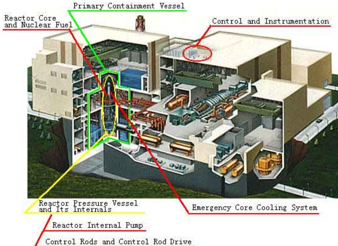
**Figure 8. ABWR Power Plant Structure**
