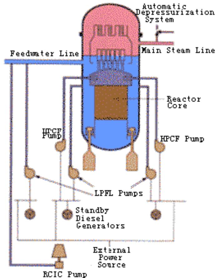
Figure 15. Emergency Core Cooling System (ECCS)
