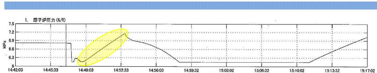
The closure of the MSIVs changed the trend of pressure inside the reactor vessel. Pressure had been trending downward as the amount of steam produced by the reactor core’s decay heat was transported through the steam pipes to the turbine. When the MSIVs closed, the steam had no place to go. Bottled up inside the reactor vessel, the continued production of steam caused the reactor vessel pressure to steadily increase for the next five minutes.
