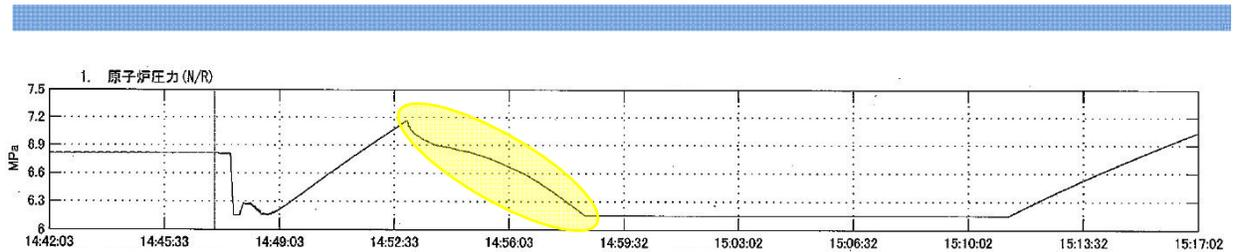
The in-service isolation condenser provided some place for the steam being produced by decay heat in the reactor core to go. Consequently, the steadily rising pressure trend following the MSIV closure was stopped and a steadily decreasing pressure trend begun. The decay heat produced by the reactor core was being used to warm the water inside the isolation condenser instead of pressuring the bottled-up volume inside the reactor vessel.
