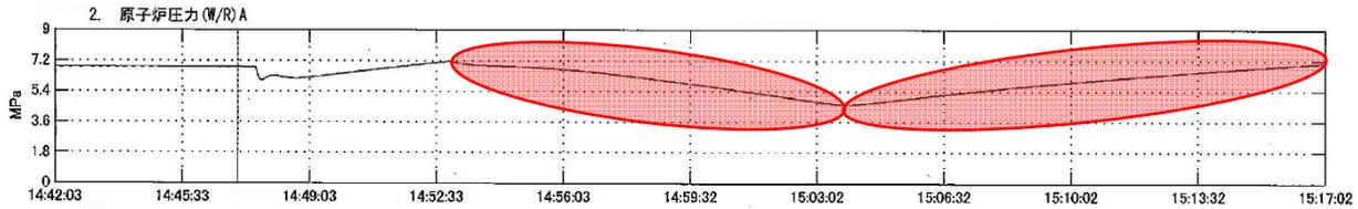
The above chart of pressure inside the reactor vessel over the wider range of 0 to 9 MPa (0 to 1,305 psig) shows that the steadily decreasing pressure trend stopped around 3:04 pm and became a steadily rising pressure trend.
