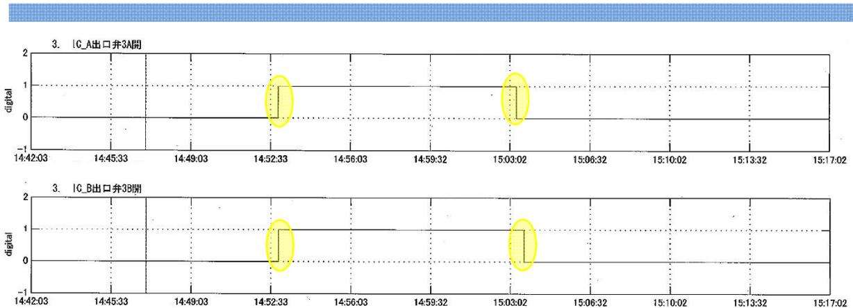
The above two charts show the logic for isolation condensers A and B. The charts show that both isolation condensers were placed in service at the same time around 2:53 pm and that isolation condenser A was taken out of service shortly before isolation condenser B at around 3:04 pm. The concurrent initiation times suggests that both isolation condensers automatically responded to the same sensed condition. The staggered termination times suggests manual action consistent with reported events.
