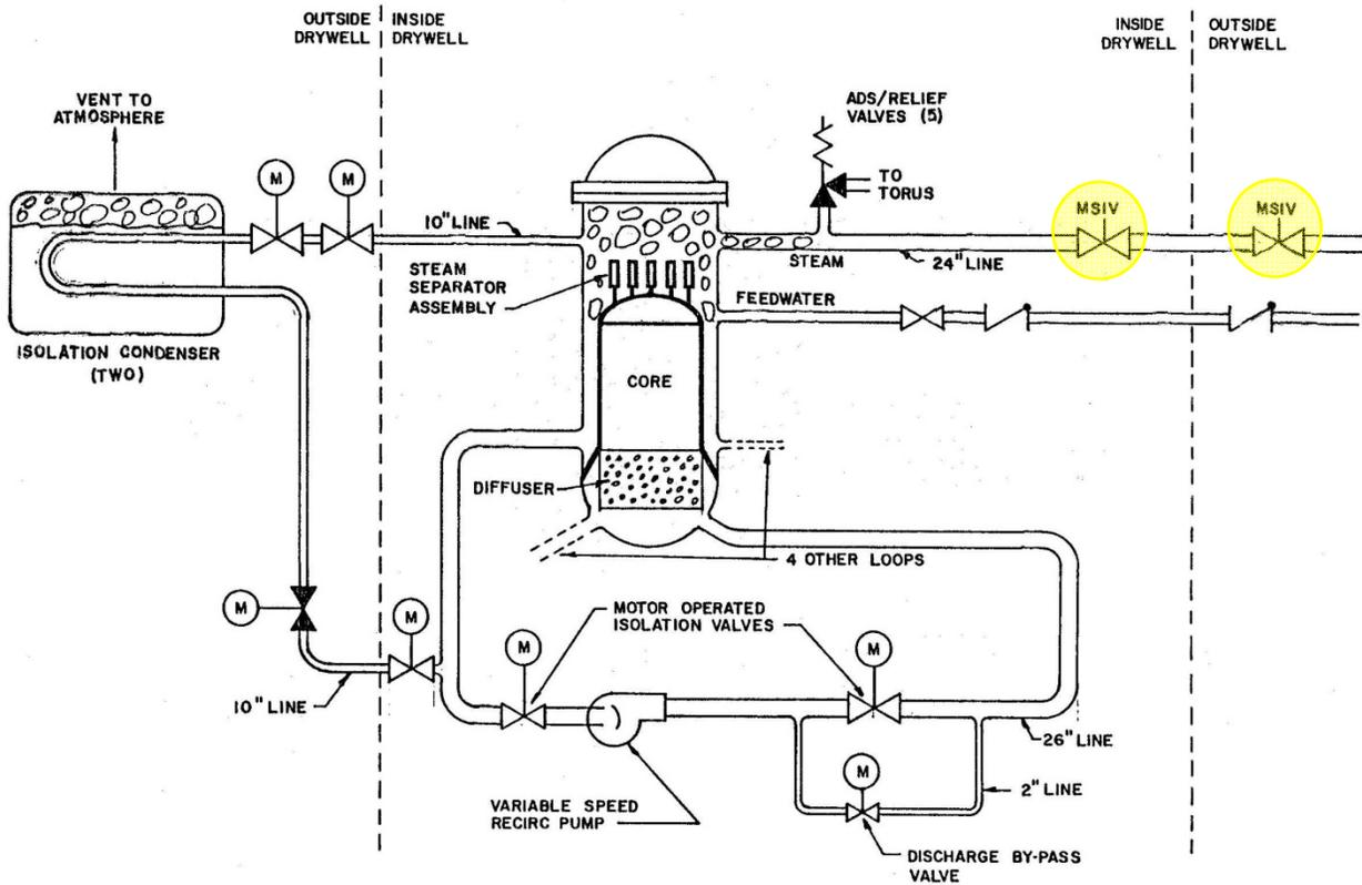
The momentary loss of power closed the main steam isolation valves (MSIVs). As shown in the diagram above, there are two MSIVs in each of the four pipes carrying steam from the reactor vessel to the turbine. The fail-safe position of the MSIVs is closed. When power was lost, the MSIVs closed. Steam being produced by the reactor core's decay heat had been traveling through the steam lines to the turbine.
