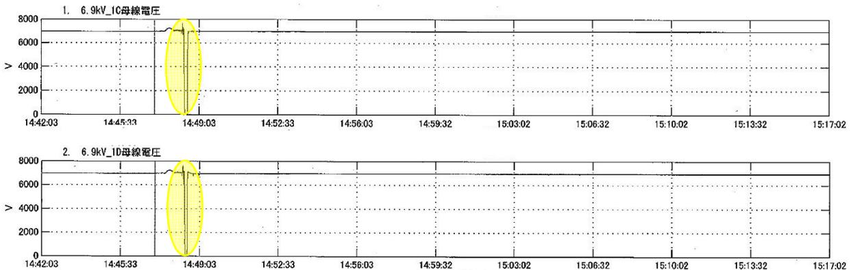
The two charts above show the voltages on 6.9 kilovolt electrical buses 1C and 1D. The plots show the brief power interruptions between the time that the turbine was tripped to stop the supply from the generator's output and the circuit breakers for the emergency diesel generators closed to restore the power supplies.
