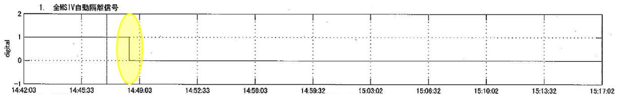
The chart above shows the digital signal for the MSIVs. A “1” indicates the MSIVs are open while a “0” indicates they are shut. When the power supply was interrupted, the MSIVs automatically closed.
