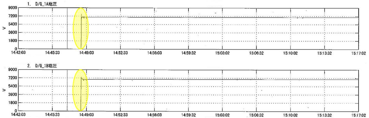
The two charts above show the voltages generated by emergency diesel generators 1A and 1B. These emergency diesel generators automatically started when undervoltage was detected on 6.9 kilovolt buses 1C and 1D and provided backup power when the normal power supplies were lost.
