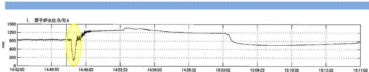
The water level inside the reactor vessel is the third key parameter. The chart above plots the water level over the narrow range of 0 to 1,500 millimeters (mm). The water level had been steady at 949 mm (37.4 inches) prior to the earthquake.
