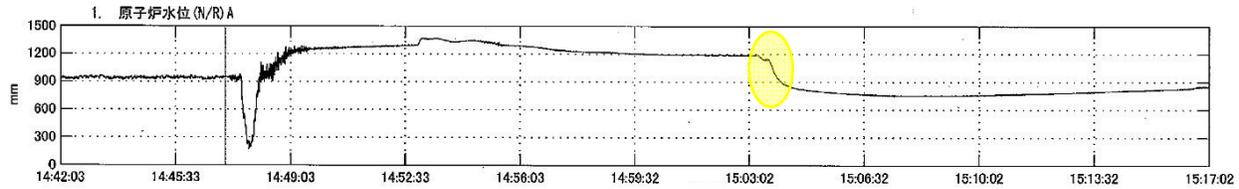
Around 3:04 pm, a significant downward step change in the reactor vessel water level occurred as shown in the chart above. The level dropped from 1,200 millimeters (47.2 inches) to around 800 mm (31.5 inches) in less than a minute. Typically, such downward step changes in water level are explained by:
